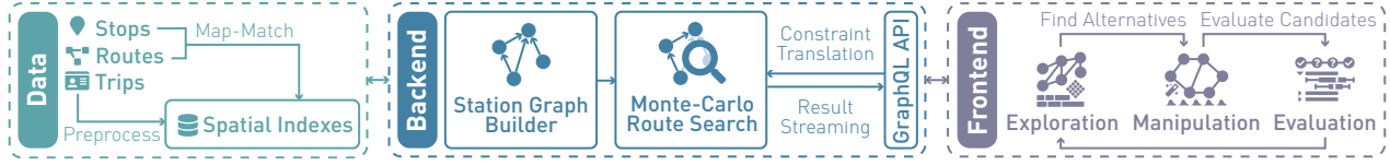
Fig. 3. The system architecture of BNVA. BNVA comprises three parts, including data storage, backend, and frontend. Data storage preprocesses the data and indexes the data with a spatial database. Backend builds station graphs and answers route generation requests. Frontend combines the exploration, manipulation, and evaluation interfaces to establish an iterative workflow for analyzing and improving the performance of bus networks.
